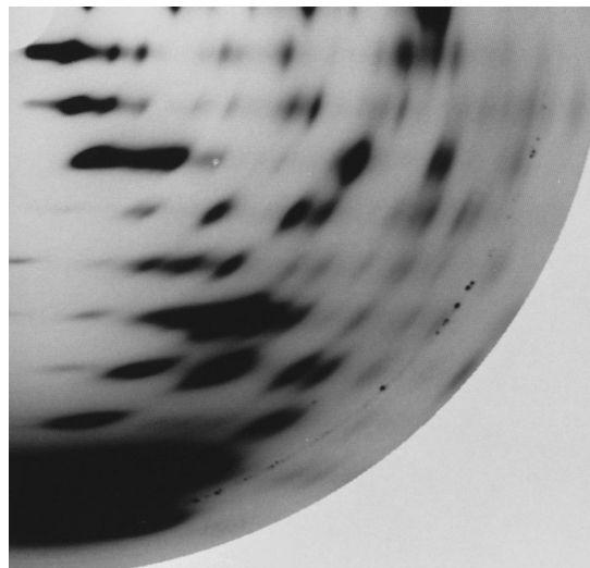
Fig. 10. Final dataset obtained by merging all of the diffraction patterns recorded during the tilt series. The ‘blind region’ is essentially non-existent.
